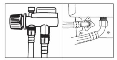
Your dishwasher comes equipped with a 'quick-connect' assembly (includes inlet and drain hose). The faucet adapter must be installed on the faucet before you can connect the dishwasher. This adapter is included inside your dishwasher.
